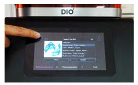
I Press the **shut down button** on the top left of the screen.
