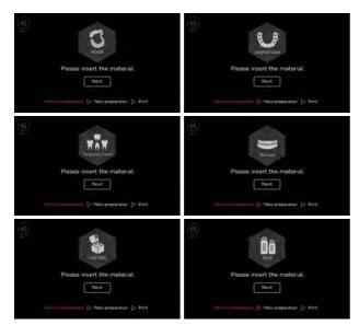
I Pour appropriate material into the vat for the printing.I Press the next button to continue.
