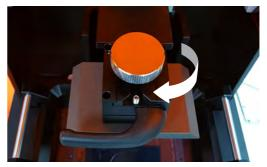
Insert the build Plate into the groove of fastening plate
