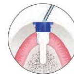
X With the needle tip not all the way down to osteotomy it is hard to irrigate
